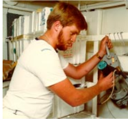
Figure 5. XBT (Expendable bathythermograph) launching
